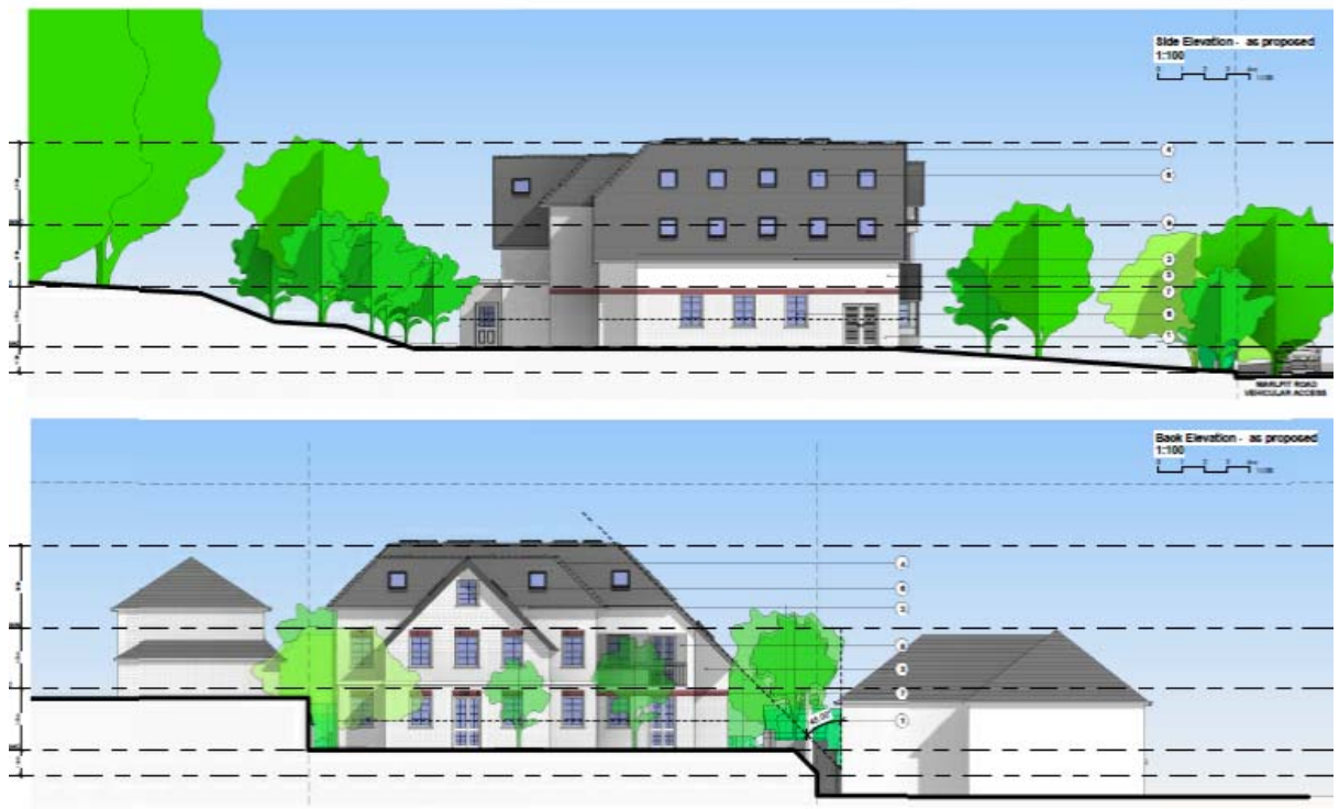
Fig 5: Proposed side elevation and rear elevation showing the change in levels
